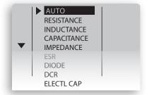
**AUTO MODE:** Select AUTO mode (AM sign appears at the in the top row of the display) for automatic measurement of inductance, capacitance or resistance.
