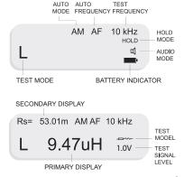
**PRIMARY DISPLAY:** The Primary Display is located in the middle of the screen and uses the largest font. It shows the dominant impedance parameter reading typically with 5 digits displayed.
