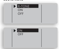
Sound menu is used to change the sound setting for measurement confirmation.
